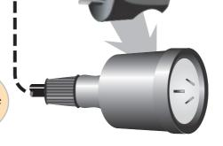
The three pin socket is the power output from the switch. Plug in whatever equipment is to be switched on and off but do not exceed the 600 watt limit.
